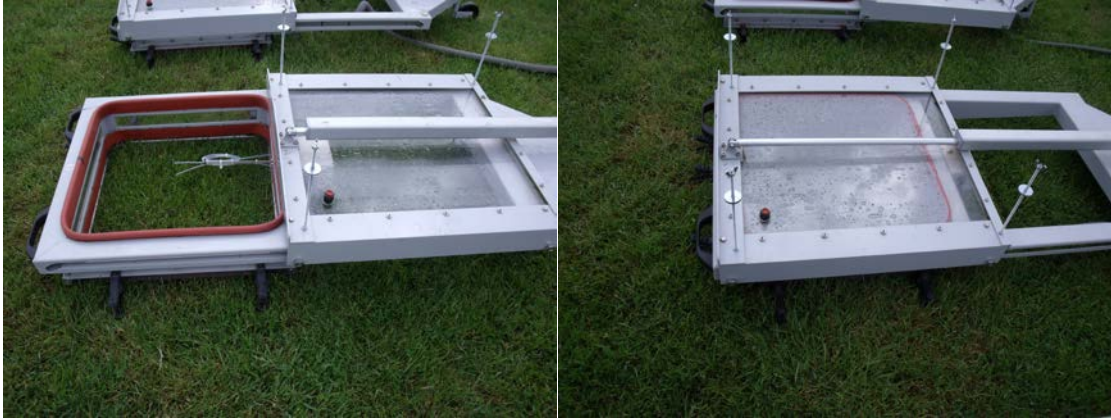
Figure 5.4: Automated chambers developed by AgResearch (New Zealand). Chamber open (left) and closed (right)
